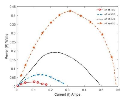
Fig. 3. Mathematical analysis of the maximum power point effect of full load tests at four different  $\Delta T$  on the output load power (P) connected to the variable load resistor (R<sub>L</sub>) when R<sub>L</sub>=R<sub>e</sub>
