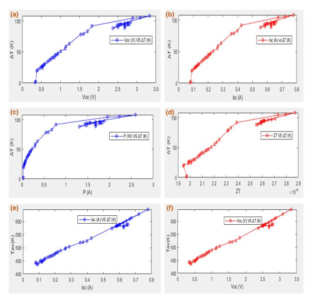
**Fig. 5.** Experimental results of the TEG-setup with natural solar thermal concentrated heat harvesting showing (a)  $V_{oc}$  versus  $\Delta T$ , (b)  $I_{sc}$  versus  $\Delta T$ , (c)  $\Delta T$  versus P, (d)  $\Delta T$  versus ZT, (e)  $I_{sc}$  versus  $T_{av}$  and, (f)  $T_{av}$  versus  $V_{oc}$
