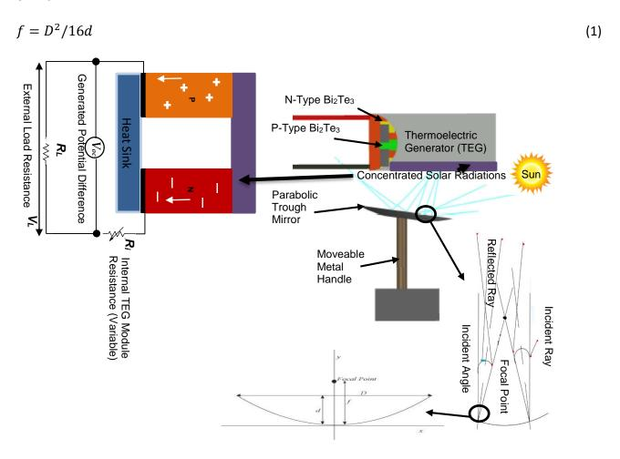
**Fig. 1.** Schematic diagram of parabolic trough mirror as a solar thermal concentrator to Thermoelectric Generator (TEG) consists of N and P and type Bi₂Te₃
