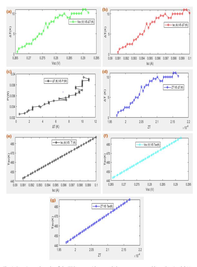
**Fig. 4.** Experimental results of the TEG-setup with quartz-halogen concentrated heat showing (a)  $V_{oc}$  versus  $\Delta T$ , (b)  $I_{sc}$  versus  $\Delta T$ , (c) P versus  $V_{oc}$  versus  $V_{oc}$  versus  $V_{oc}$  versus  $V_{oc}$  and (g)  $V_{av}$  versus  $V_{oc}$  versus  $V_{oc}$
