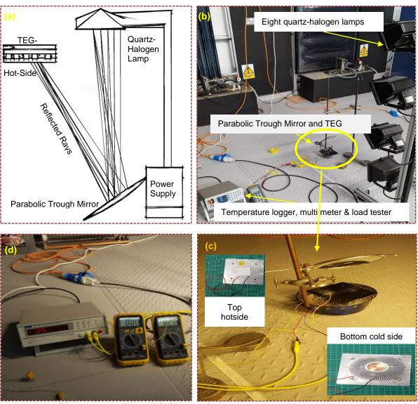
**Fig. 2.** Experimental TEG-setup with quartz halogen radiative concentrated heat testing components showing (a) projected sketch matching the focal length, (b) four quartz halogen lamps positioning in achieving concentrated temperatures (c) on the hot side of the TEG whilst the cold-side submersed with ice-cubed container and (d) connected to live measurement digital meters
